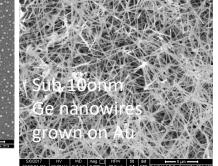
Vapor transport growth of Ge nanowires on Au catalyst Dense array of TiO<sub>2</sub> nanowires grown by Hydrothermal growth on FTO substrate
