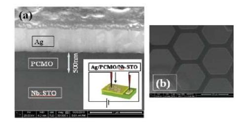
Junction of Ag/PCMO/NbSTO multilayer film grown by PLD and then covered with patterned. Ag pads
